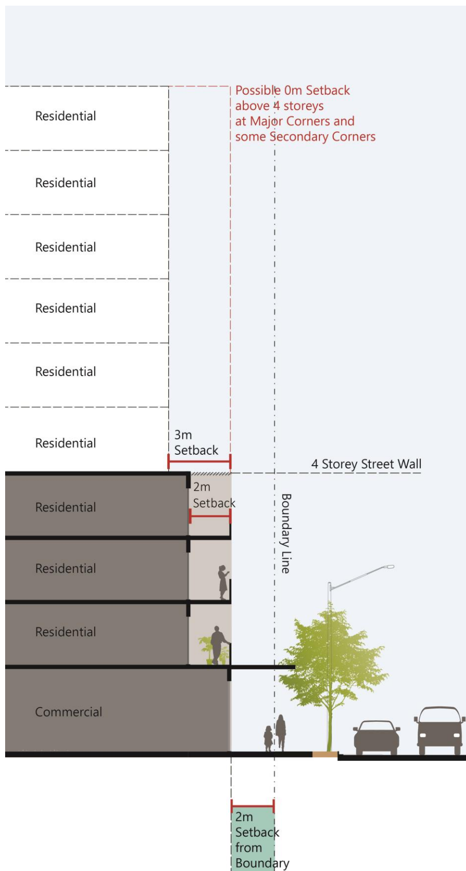
Figure 4: Setbacks on identified corners
