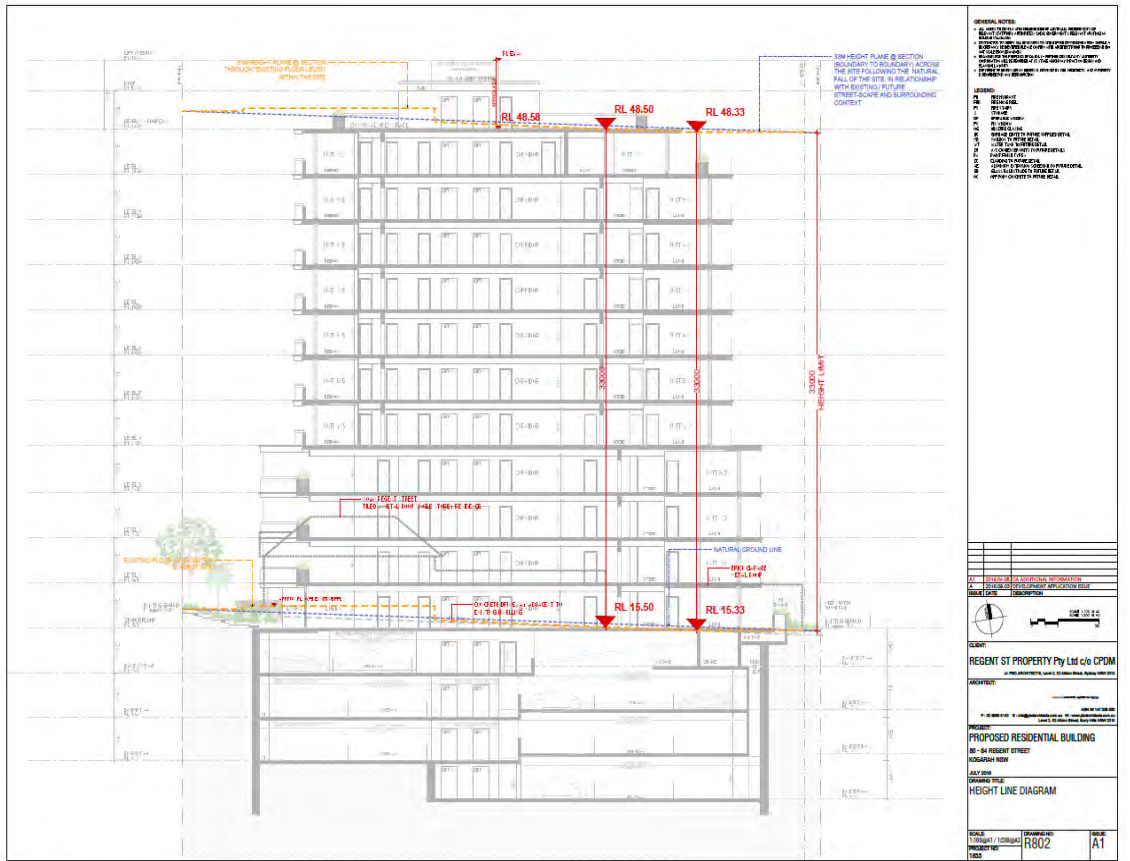
Figure 3:Section showing height breach (Source: PBD Architects)
