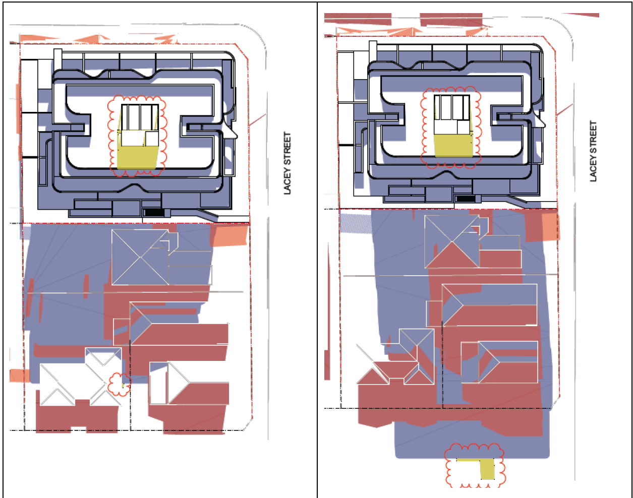
Figure 3 Shadow diagrams detailing the extent of the non-compliance at 9am, 12noon, 2pm and 3pm
